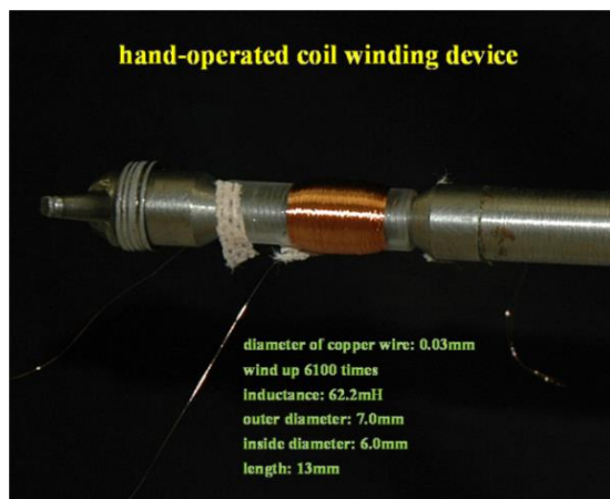
Fig. 2. Hand-operated coil, 0.03mm copper 6100 times.
